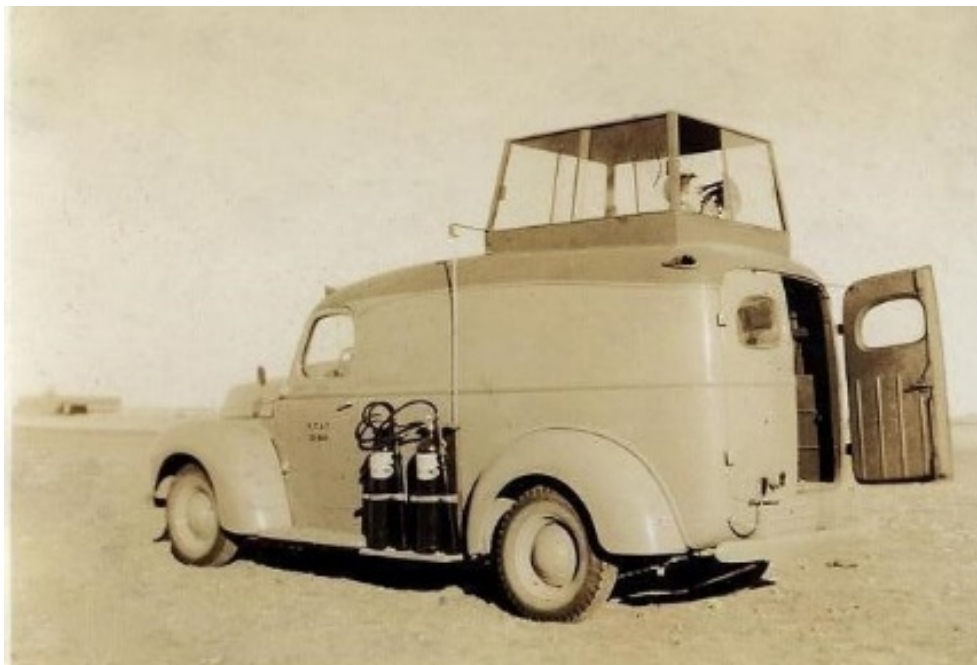
The RAF mobile control tower airmen sending lamp signals to the Harvard pilots, [no aircraft radios] with the Airdrie hangar and main control tower in the background. The bright red painted roof clearly shows in this image. RCAF and serial number 31-129 in black are stenciled on yellow driver/passenger doors.
