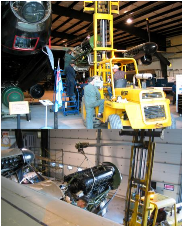
Shop volunteers are seen here reinstalling the overhauled, port inner Merlin engine as of August 9. The propeller is still being checked over by Canadian Propeller Ltd. and will be back on the engine some time this coming winter.
