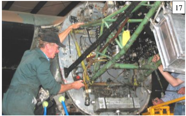
Brian Taylor fastens the mount bolts that hold the Merlin engine to the firewall.
