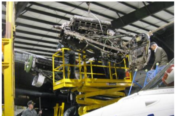
Brian Taylor fastens the mount bolts that hold the Merlin engine to the firewall.
