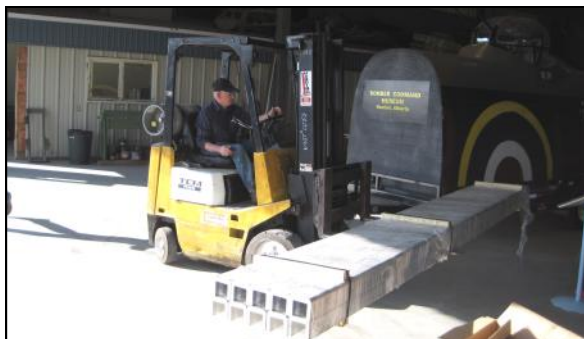
Bob Evans uses a forklift to place new extruded aluminium beams, made for use in restoring Halifax centre-sections. Sprung Building Industries Ltd. , Aldersyde, AB. had these made for the project. THANKS to Phil Sprung, his family and employees.
