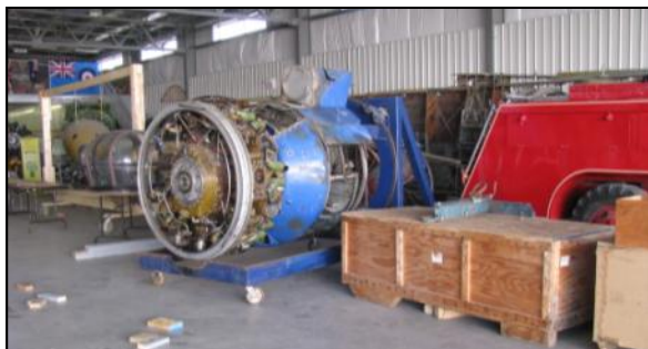
One of four Hercules engines complete with rotating stand; more parts in the big box.
