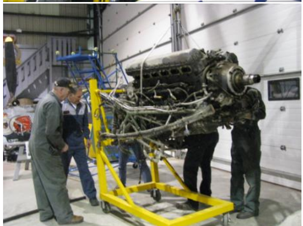
The Lancaster's #1 Merlin being removed from its position on the port wing. It is the Lanc's last engine to go into the museum shop for overhaul. It should be back on the Lanc and running by the summer of 2013.
