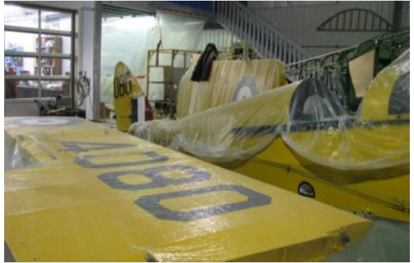
Photo shows the completed starboard lower wing in the foreground and in the rear the two upper wings standing on edge with the fuselage between. As this newsletter goes to print only the port lower wing remains to be painted.
