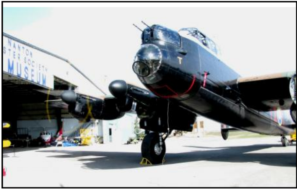
Bomb bay doors are shown here completely closed using the aircraft hydraulic system at the trial running of the Merlin engines on April 17. Closed hydraulically for the first time in sixty-some years.
