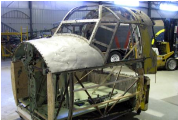
Anson cabin stripped and modified for installation of the simulator electronics and mounted on a castor base. April 20 photo.
