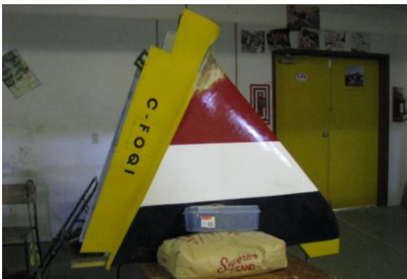
Repairs to the vertical fin are underway.
