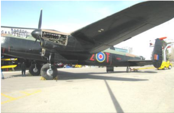
With the two Merlins running on April 17, the flaps were articulated. Here they are shown in the full up position.
