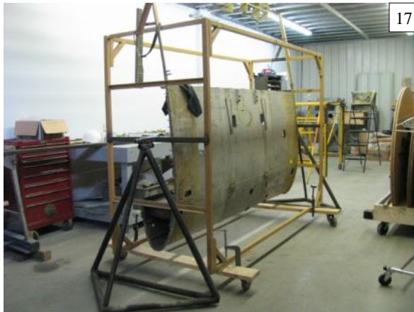
The Yale centre-section is seen here in a jig that is being modified so it can be rotated. This will make the leading edge more easily assessable for the necessary repair work to take place. A new main spar and other components are now in the works.
