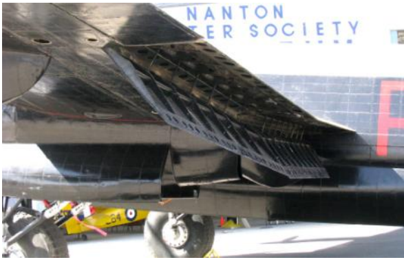
This photo shows the flaps in their full down position during the April 17 engine run, using the refurbished hydraulic system.
