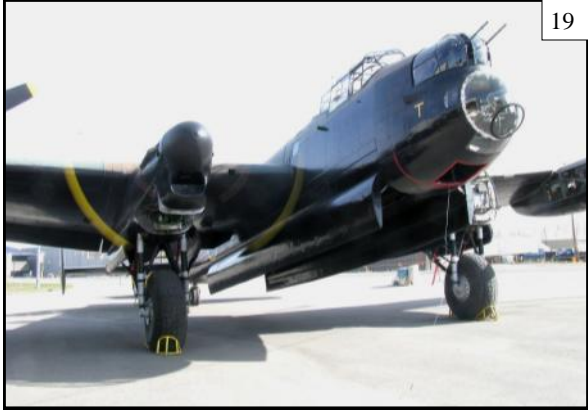
The bomb bay doors are shown here fully open, testing the hydraulic system with the Lanc outside and the Merlins running in mid-April at the trial run to make sure everything was ready for the scheduled summer event run-ups.
