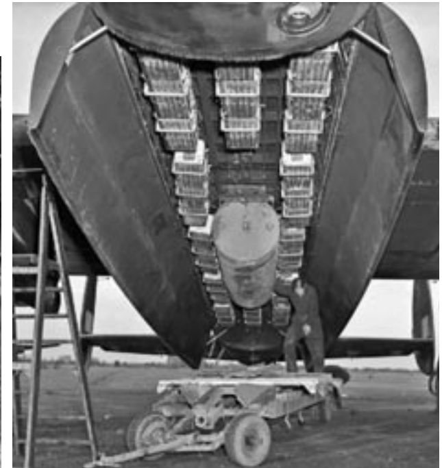
A Lancaster bomb-bay loaded with a high-explosive, 4000 pound 'cookie' and 'small bomb containers' packed with incendiaries
