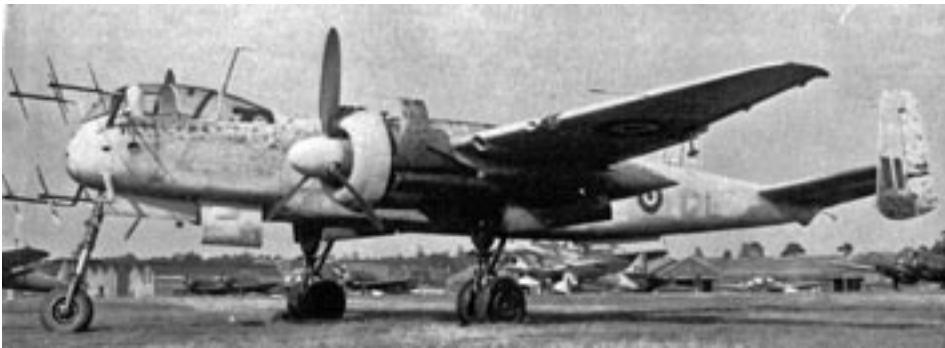
The Heinkel He 219 was known as the 'Eagle-Owl'. A relatively sophisticated design, it was the first operational military aircraft to be equipped with ejection seats and the first operational German World War II-era aircraft with tricycle landing gear. Had the He 219 been available in quantity, it might have had a significant effect on Bomber Command's operations but only 294 were built by the end of the war.
