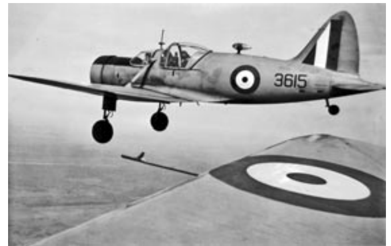
Beginning in early 1942, Fleet Forts were used at 2 Wireless School. However, the Forts made fourteen engine-related forced landings in a three month period. As well, they were under-powered given the weight of two crew members, and the heavy radio equipment. They were replaced by Harvards.
