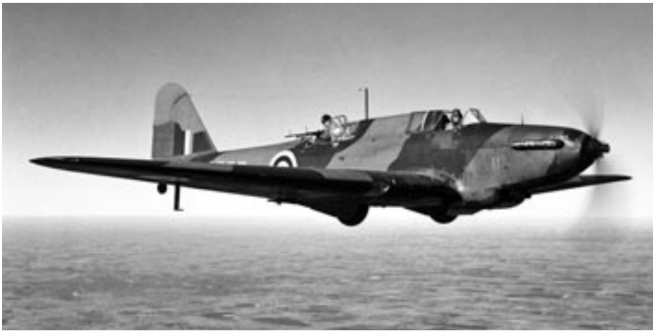
During the early years of the BCATP, Fairey Battles were used as gunnery trainers using obsolete, single Vickers guns on a flexible mounting in an open cockpit
