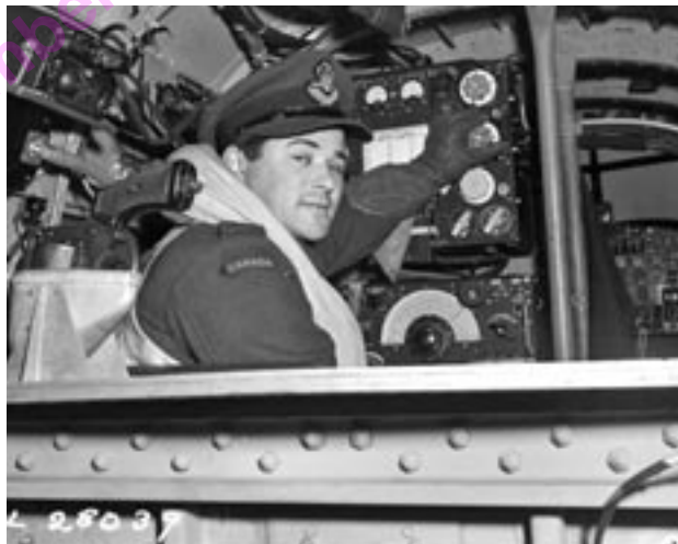
The operator in a Lancaster sat with his back to the main wing spar. Note the cockpit at right and the 'Very' flare pistol at left.
