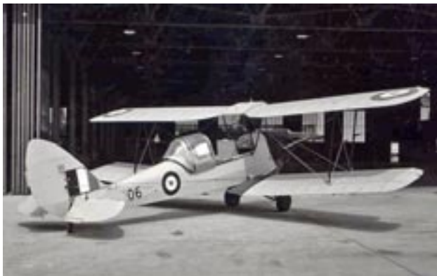
For much of the war, most student pilots learned to fly on the De Havilland Tiger Moth
