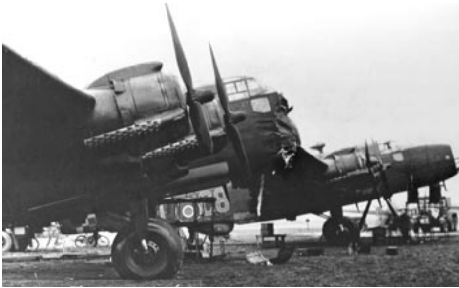
Mid-air collisions often occurred within the bomber stream, particularly at turning points on the route to the target. This Halifax had about nine feet of its nose section chopped away in an aerial collision. F/O A.L. Wilson lost his navigator and bomb aimer, both of whom were at their stations in the nose.
