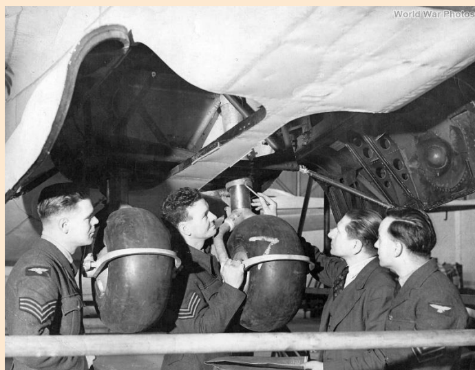
TWIN TAIL WHEELS ON STIRLING
